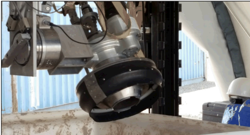
Figure 14. Hanford Waste End Effector Tilt Mechanism.
