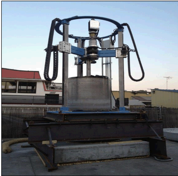
Figure 16. Example Rotary Core Cutter.
