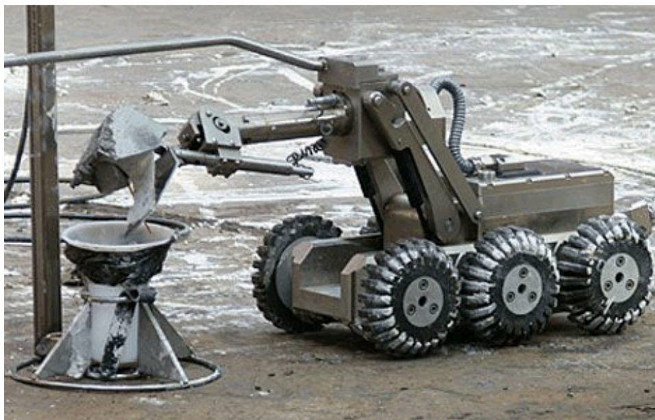
Figure 5. Current Crawler and Sample Scoop Device.
